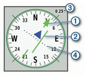
The course pointer ① indicates your relationship to the course line leading to the destination. The course deviation indicator (CDI) ② provides the indication of drift (right or left) from the course. The scale ③ refers to the distance between dots ④ on the course deviation indicator, which tell you how far off course you are.
