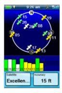
The Satellite Status screen displays a graphical representation of the satellites overhead in relation to you current location (the center of the circle) The color of the satellite graphics, as well as the bar graph, indicate the signal strength of the signals being received. The numbers indicate the assigned satellite designation. The data fields at the bottom of the display are customizable (see *Customizing the Data Fields*).
