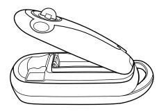
Install two AA batteries as shown.
